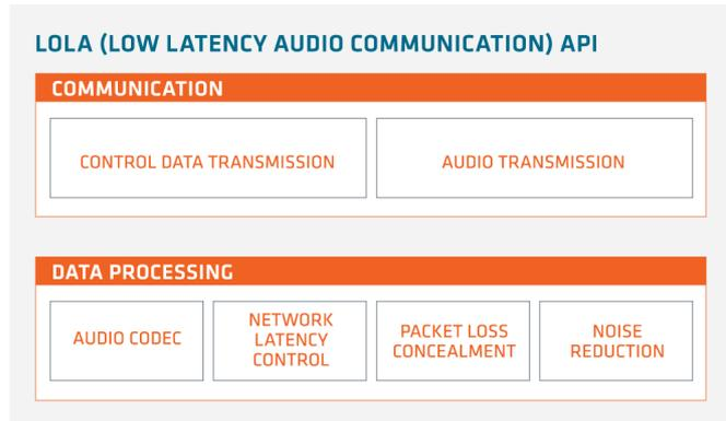
**Jacoti Lola** is a new Wireless Protocol implemented with the goal of having Low Latency Audio Communication applications work effectively on off-the-shelf devices and network infrastructures; hence allowing to bring this technology to end-users for a fraction of the price of other equivalent technologies without compromising latency, quality or signal-to-noise ratio.
